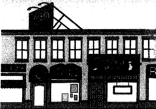
This arrangement of signs blocks building elements and creates an image of visual clutter.
